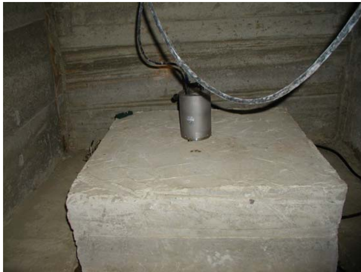
Photo. 2 Georgian Seismic Network. Seismometer on plinth in vault at end of tunnel in Photo. 1.
